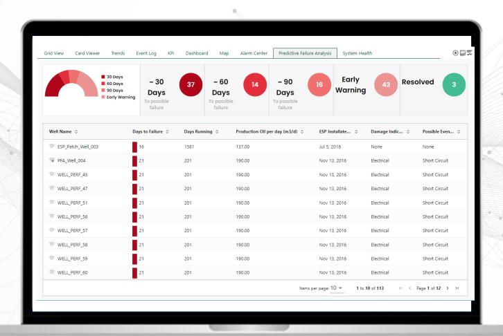
Digital solution to leverage state-of-the-art artificial intelligence/machine learning and physics-based models to detect operational events and anomalies in your ESP system early-before a costly failure
